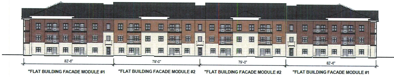
BUILDING ELEVATION - EAST (MAJOR FACADE = 100% STONE & BRICK VENEER)
