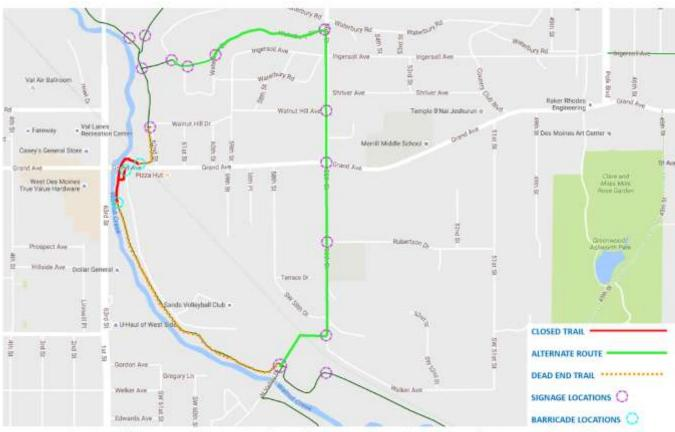
Detour signage and markings shall be consistent with the Manual on Uniform Traffic Control Devices (MUTCD) and shall be installed and maintained by City of West Des Moines.
