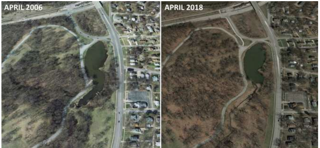
MacRae Pond – siltation over time
