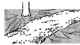
Figure 6. A root system bridge will help protect trees in the path of construction vehicles.
