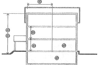
Figure 135-2.16-C. House D Building: Height and Use Requirements
