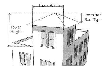
Figure 135-2.20-C. Example of a Tower
