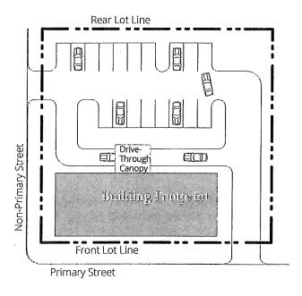
Figure 135-2.22-C. Example of Drive-Through Facility Layout.
