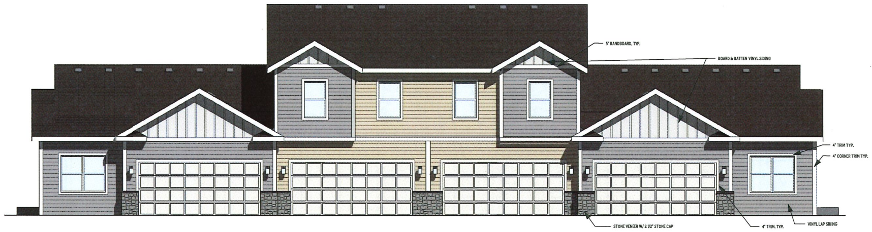
② REAR ELEVATION - Color Elevation 1/8" = 1'-0"
