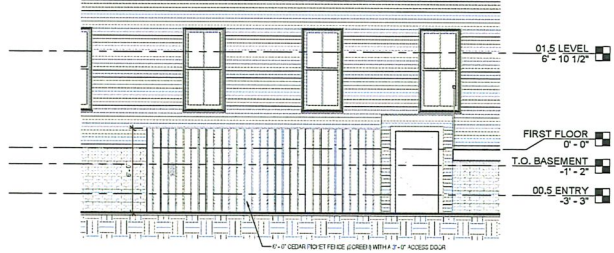
6 | EXT ELEVATION - NORTH MECHANICAL SCREEN WALL 1/4" = 1'-0"
