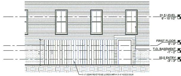
6 | EXT ELEVATION - NORTH MECHANICAL SCREEN WALL 1/4" = 1'-0"
