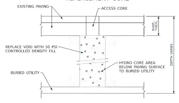
SPECIFICATION FOR THE CONSTRUCTION OF PAVEMENT CORE RESTORATION
